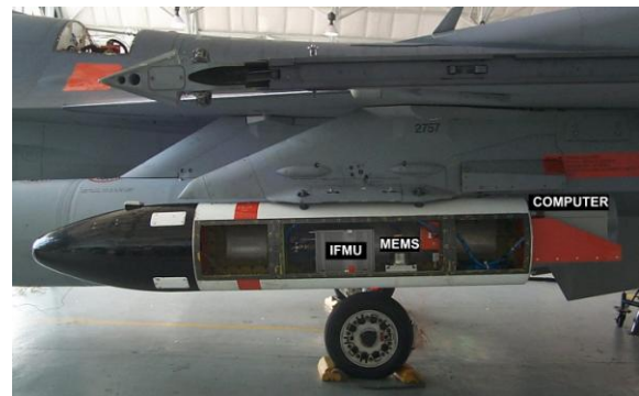
Figure 5.1-1 MICA Equipment in GI Pod
